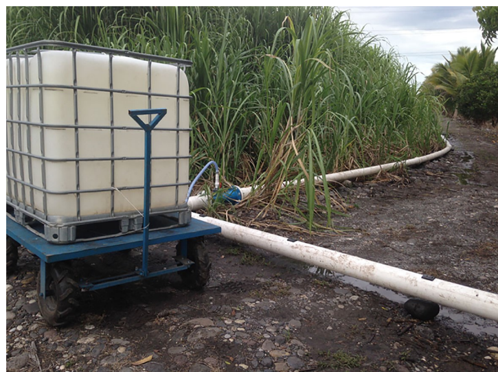
Figure 7. Field tests of the fertigation system on land cultivated with sugarcane ( Saccharum spp. hybrid) var. Mex 69-290.
