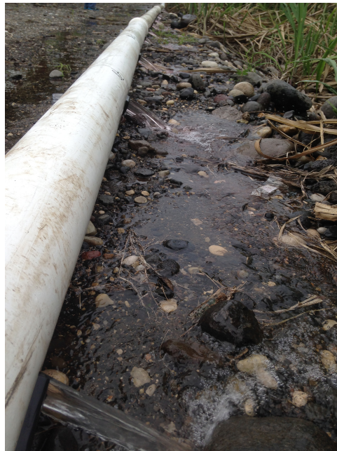
Figure 1. Multi-gates in a low-pressure irrigation system in sugarcane ( Saccharum spp. hybrid) var. Mex 69-290.
