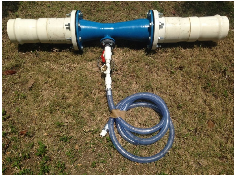
Figure 6. Venturi injector used for fertigation in the low-pressure irrigation system with multi-gates in sugarcane cultivation ( Saccharum spp. hybrid) var. Mex 69-290.
