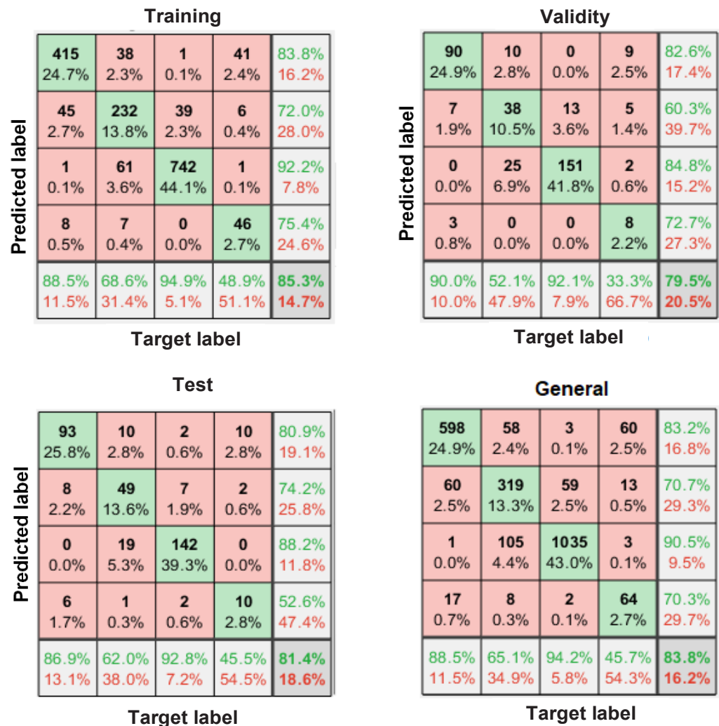
Figure 5. Confusion matrices of the Multilayer Perceptron (MLP) Neural Network for each stage of development ( 86 \times 50 \times 50 \times 4 ).
