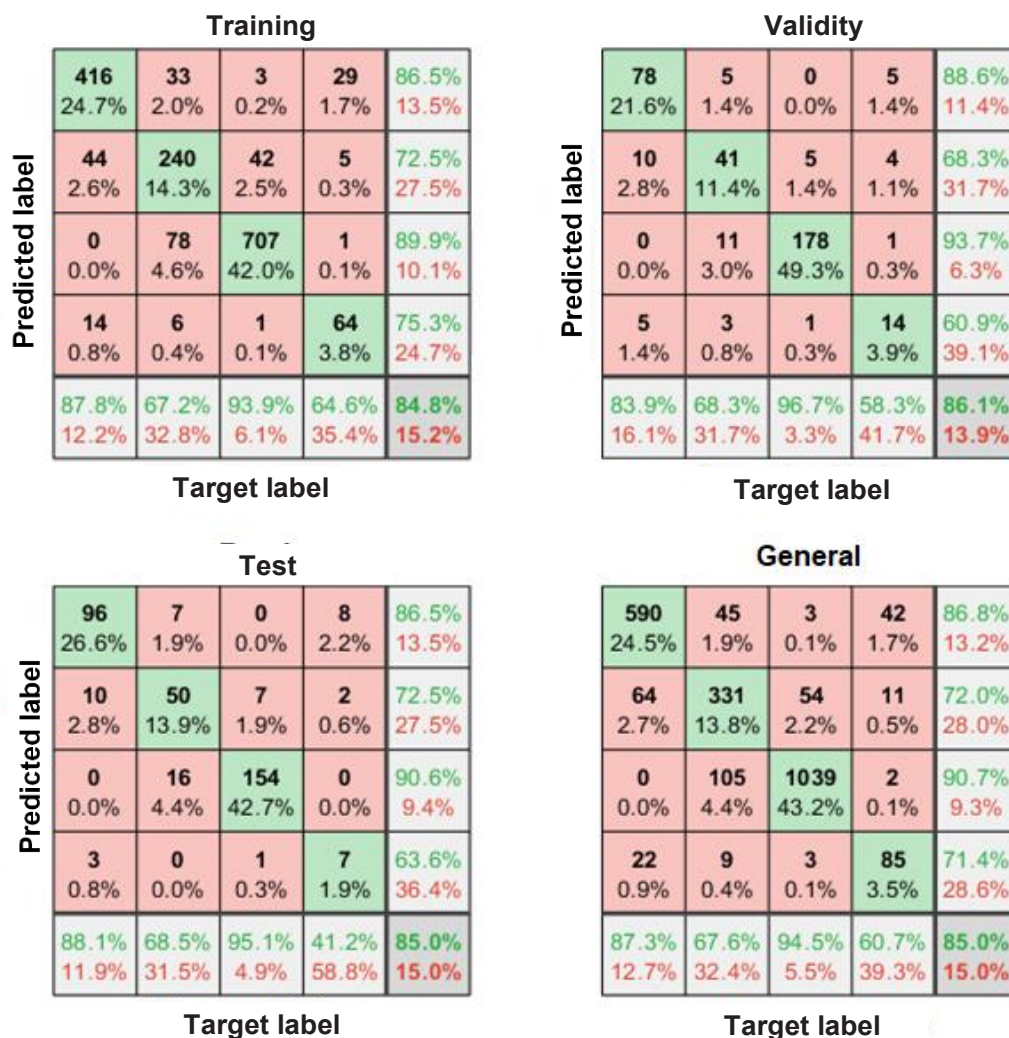
Figure 6. Confusion matrices of the Multilayer Perceptron (MLP) Neural Network for each stage of development (29 × 50 × 50 × 4).
