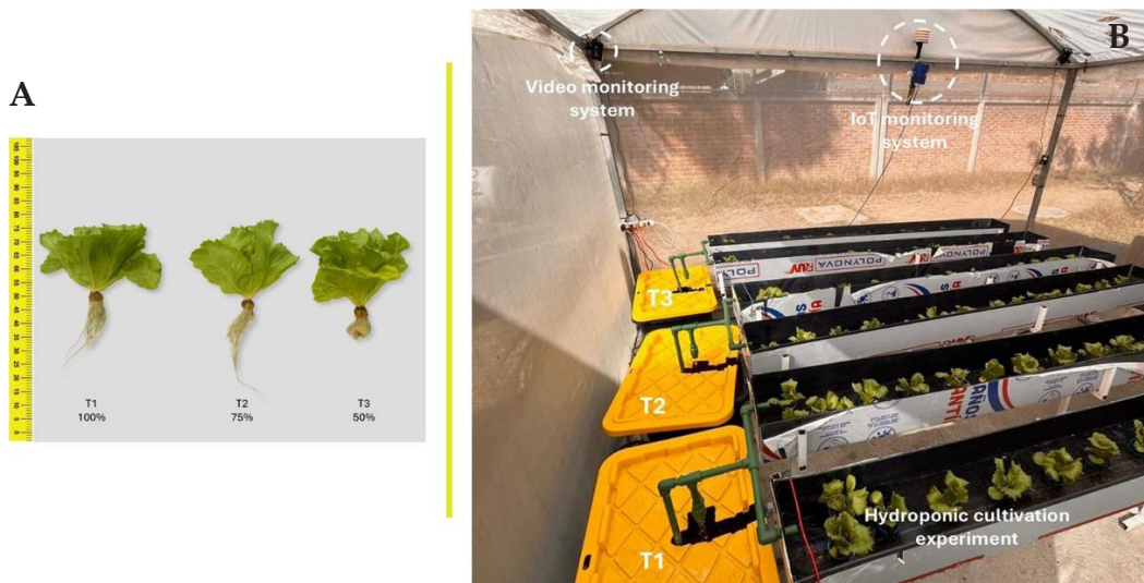
Figure 3. Experimental setup of the hydroponic greenhouse showing the arrangement of nutrient treatments T1 (100 %), T2 (75 %), and T3 (50 %), the IoT monitoring unit, and the video monitoring system used for data acquisition and environmental control.
